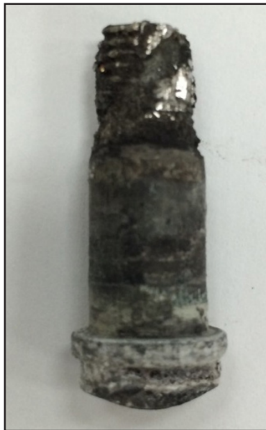
HARDENED WHITE SUBSTANCE COATING MAJORITY OF INTERIOR BODY, STEM, BALL & SEAT DAMAGED BEYOND REPAIR
